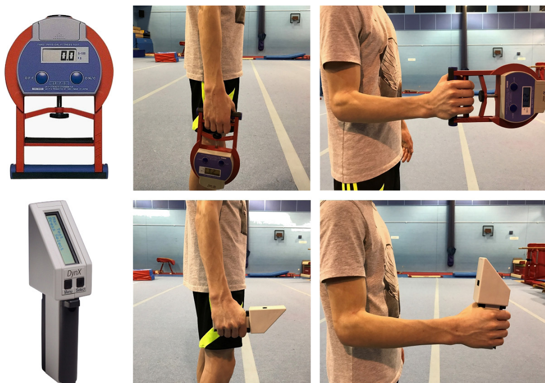
Fig. 1. Handgrip strength test with fully extended and flexed elbow, using TKK (above) and DynX (below) dynamometers
